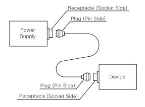
Connector combinations are formed with plugs and receptacles that are connected with pin and socket contacts.
